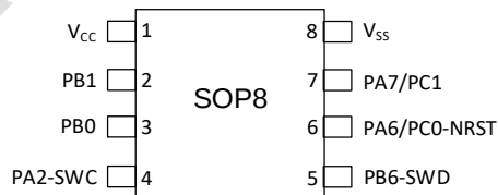
图 3-3 SOP8 Pinout1 PY32F002BL15S6-C (Top view)
